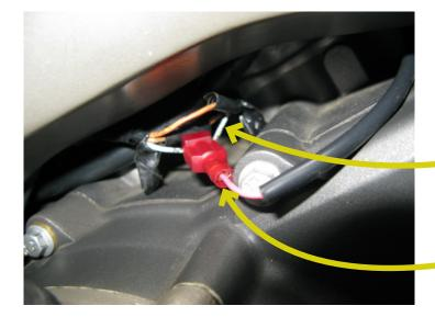
Then insert the Bazzaz SPD connector (red connector with pink wire) into the scotchlok.
