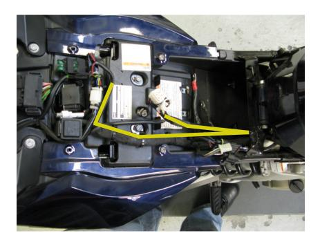
6. Now locate the factory TPS connector inside the airbox (at the rear). Crimp a supplied Scotchlok onto pin 1 (as numberd on back of the factory connector) of the rear TPS connector. Insert the Bazzaz TPS connector (red connector with blue wire) into the Scotchlok.
