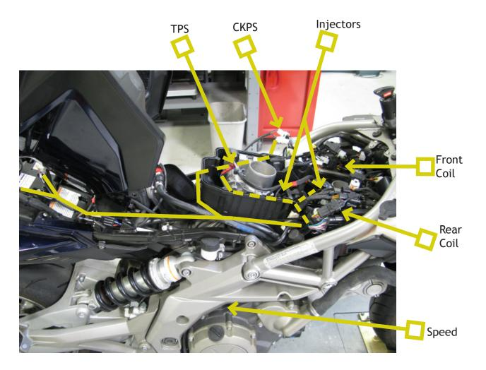
5. The remaining section of the wiring harness will route under the tank and through the battery tray, to the tail of the bike.
