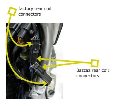
15. Route the rest of the coil harness around the front of the airbox.
