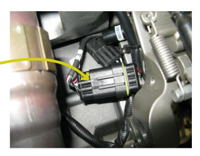
14. Now connect the Bazzaz coil harness main connector to the control unit.
