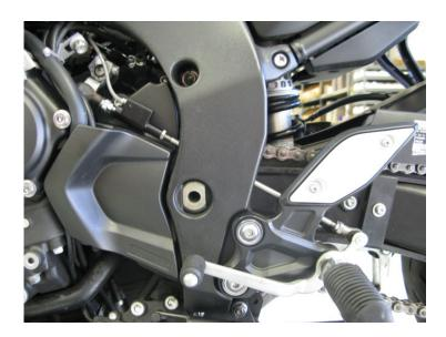
13. Next you will need to disconnect the Factory **O2 SENSOR**. The O2 sensor connector is located on the left side of the engine compartment, and can be located by tracing the wire up from the O2 sensor on the left side of the exhaust collector. This sensor will no longer be used; the wires should be neatly secured away from any moving components, or the sensor may be removed and the remaining port/bung in the exhaust can then be plugged.
