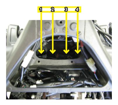
12. Now you will begin the installation of the **SHIFT SWITCH** by removing the factory shift rod. Next install the Bazzaz shift switch onto the front inkage, then install the supplied **SHIFT ROD** between the rear linkage and the shift switch. Adjust the foot pedal to preferred height and secure components by tightening the 10mm nuts. Now route the shift switch connector up to the mating connector on the Bazzaz coil harness.
