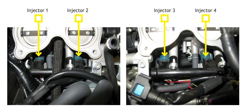
9. Route the remaining potion of the Bazzaz fuel harness with the TPS (Throttle Position Sensor) connectors around the right side and to the front, middle of the throttle bodies. Locate the factory TPS connector in this area and disconnect it from the sensor. Install the Bazzaz TPS connectors inline between the factory connector and sensor.
