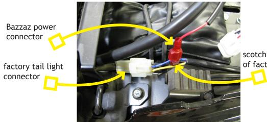
scotchlok crimped onto blue wire of factory tail light connector
