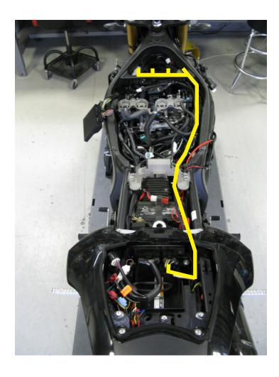
11. From **right** to **left**, unplug the factory coil connectors from the stick coils. Plug the Bazzaz **COIL** connectors inline between the factory connectors and stick coils. Start with the Bazzaz coil connectors with the green wires.
