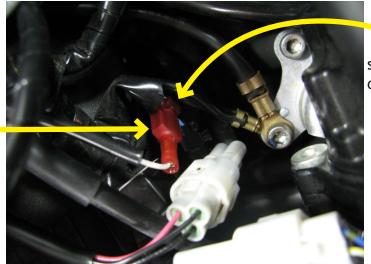
scotchlok crimped onto blue wire of factory neutral connector
