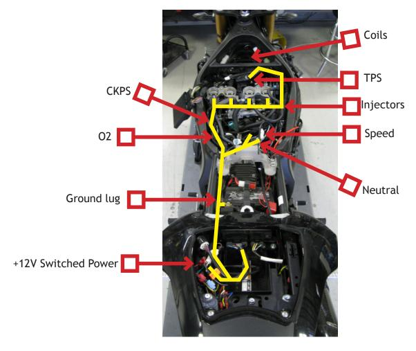
3. Locate the factory tail light connector in the left side of the tail section. Crimp a supplied scotchlok onto the middle **blue** wire of the factory connector and insert the Bazzaz **POWER** connector (orange label on lead) into the scotchlok.
