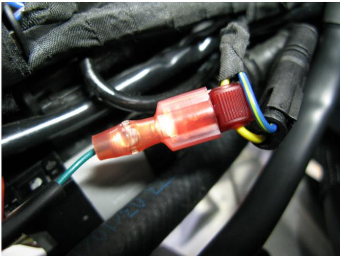
C) Crimp a supplied scotch-lok connector onto the **white/gray wire** on the factory Throttle Position Sensor connector at pin location 2. Insert the mating T-tap connector of the Bazzaz harness containing the **blue wire**.
