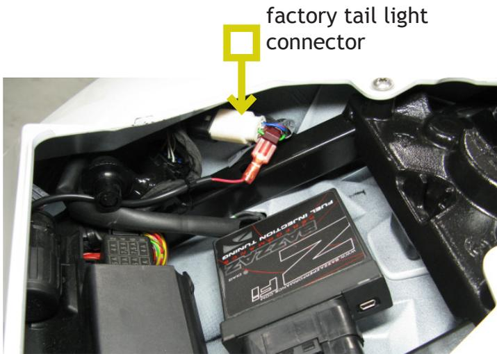
3. On the factory harness, locate the **green wire** of the tail light connector. Crimp a supplied scotch-lok connector onto the **green wire** and insert the mating T-tap connector of the Bazzaz harness identified on page one of these instructions as “Power” (**red wire**).
