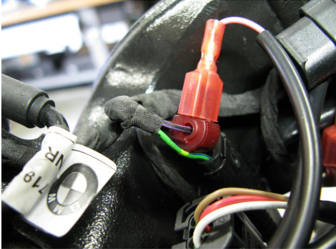
B) Crimp a supplied scotch-lok connector onto the **yellow wire** of the factory Crank Position Sensor connector. Insert the mating T-tap connector of the Bazzaz harness containing the **green wire**.
