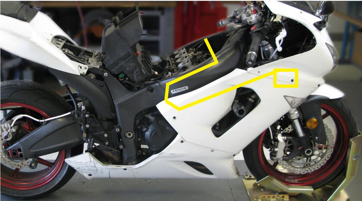
11. From **right to left**, unplug the factory coil connectors from the stick coils. Plug the Bazzaz **COIL CONNECTORS** inline between the factory connectors and stick coils. **Start with the Bazzaz coil connectors having the green wires.**
