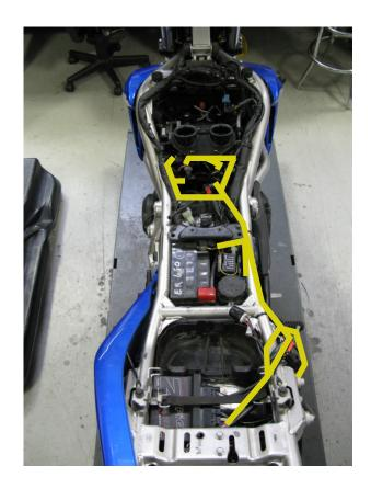
3. Locate the factory tail light connector, and crimp a supplied scotchlok onto the **red wire** of the factory connector. Then insert the Bazzaz power connector (harness lead has an orange label) into the scotchlok.
