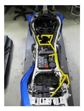
3. Locate the factory tail light connector, and crimp a supplied scotchlok onto the **red wire** of the factory connector. Then insert the Bazzaz power connector (harness lead has an orange label) into the scotchlok.
