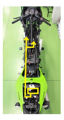
13. Locate the factory coil connectors. Disconnect the factory coil connectors from the ignition coils and connect the Bazzaz coil connectors inline with them according to the labels.
