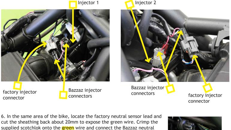
connector (red connector with white/blue wire) to the scotchlok.
