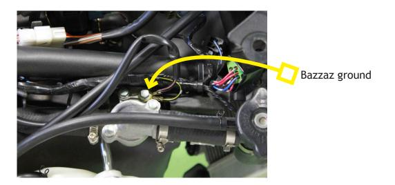
12. Now you are ready to install the coil harness. Begin by plugging the main connector of the coil harness into the Bazzaz unit. Then route the coil harness along the same path as the Bazzaz fuel harness.
