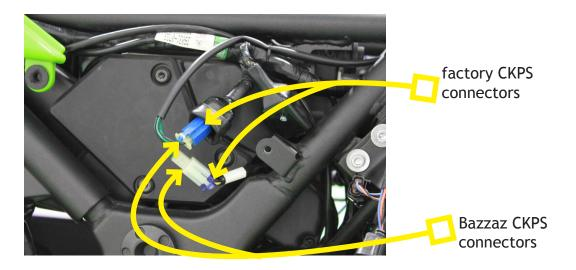
10(B). Locate the black factory CKPS connectors which are found on the left side of the air box and disconnect them. Connect the Bazzaz CKPS connectors in-line with the factory connectors.
