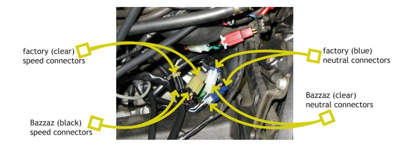
9. The red crank shaft position sensor is just above the rubber boot, next to the large grey connector; locate this and plug the Bazzaz CKPS connectors in line with the factory connectors.
