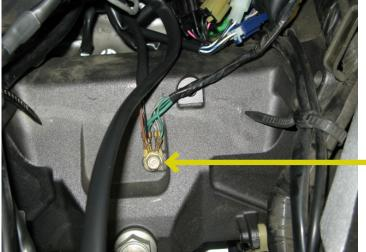
10. Locate a suitable chassis ground to attach the Bazzaz fuel harness ground lug.
