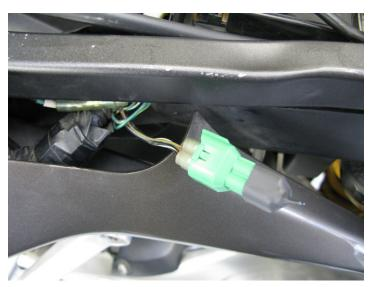
3. Place control unit in the tail compartment and route the fuel and coil harnesses' main connectors up into the compartment from the rider seat area so that the fuel harness is running along the left of the battery and the coil harness is running along the right side of the battery. Connect the harnesses to the control unit.
