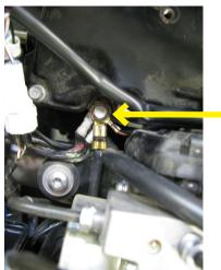
5. Next locate the factory ground lug and attach the Bazzaz ground lug to it.
