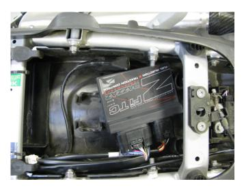
3. Connect the main connector of the Bazzaz fuel harness into the control unit and begin routing the fuel harness towards the front of the motorcycle. Continue routing the harness under the support bar and along the left side of the frame.
