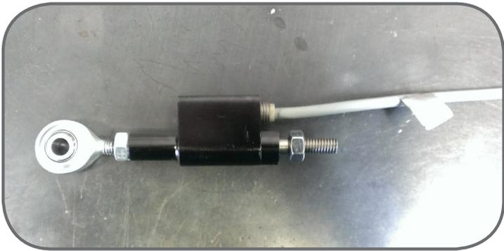
7. Using the factory bolt, secure the Bazzaz shift switch and heim joint to the shift knuckle.
