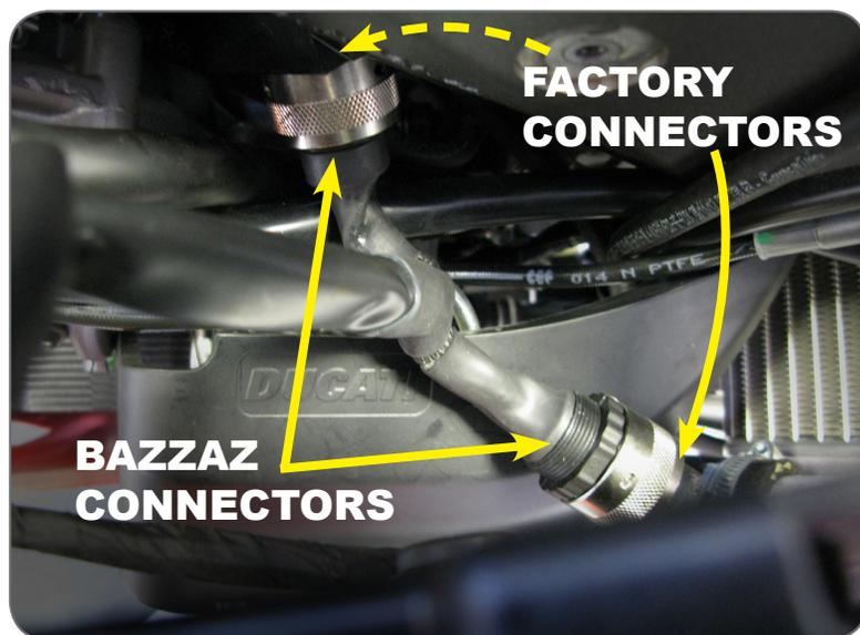
*19-pin connector is for the injectors and TPS*
