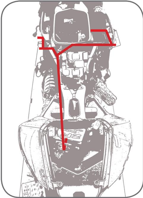
1. Connect the main connector of the Bazzaz fuel harness to the control unit.
