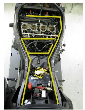
4. Locate the tail light connector on the factory wiring harness on the right side of the tail compartment, in a rubber boot between the sub-frame and fairing. Plug Bazzaz power connectors in line with the factory tail light connectors.
