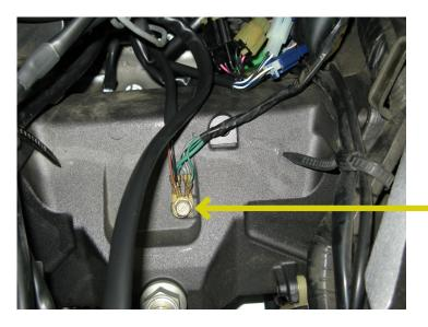
10. Locate a suitable chassis ground to attach the Bazzaz fuel harness ground lug.
