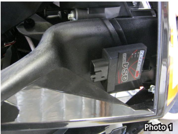
3. Connect the Bazzaz harness to the control module and begin to route it across the front of the engine. Remove the factory harness connector from the ignition coil of the front cylinder and connect the mating Bazzaz harness coil connectors inline (photo 2).
