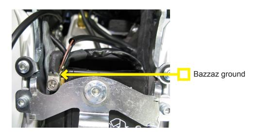
5. Now locate the factory Gear Position Sensor (GPS) connector on the left side of the frame. Crimp a supplied Scotchlok onto the **yellow/black** wire of the GPS connector and insert the Bazzaz **GPS** connector into the Scotchlok.
