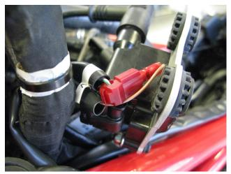
9. Route the front coil connector down the left hand side of the bike towards the factory TPS. Locate the factory coil connector. Disconnect the factory coil connector, and use the supplied scotchlok to crimp onto the factory grey/blue wire and connect the Bazzaz front coil connector. Reconnect the factory coil connector.
