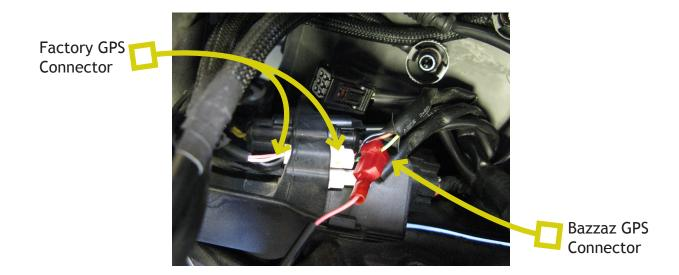
6. Continue routing the coil harness, following along with the factory harness down the left side of the motorcycle.
