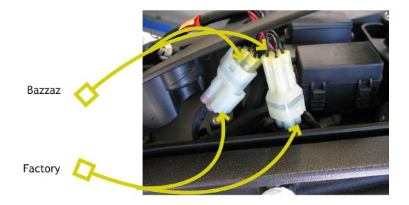
5. Locate the GPS (Gear Position Sensor) connector (small white three pin connector) near the bottom of the tank, behind the rear exhaust. Trim the wire sheathing back and crimp a supplied scotchlok onto the **yellow/green** wire of the factory GPS connector. Now insert the Bazzaz GPS connector (red connector with pink wire) into the scotchlok.
