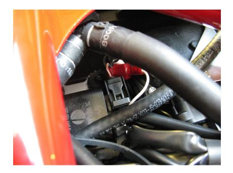
10. Now you will begin the instillation of the shift switch. Remove the stock shift rod and the heim joint attached to the shift lever. Screw the shift switch into the factory heim joint on the upper shift linkage, then screw the supplied heim joint onto the shift switch to the desired length. Last, secure the heim joint to the shift rod then secure all 10mm nuts. Route the shift switch connector up to the mating connector on the Bazzaz coil harness.
