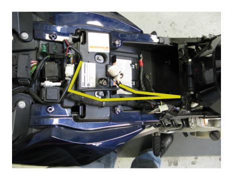
6. Now locate the factory TPS connector inside the airbox (at the rear). Crimp a supplied Scotchlok onto pin 1 (as numbered on back of the factory connector) of the rear TPS connector. Insert the Bazzaz TPS connector (red connector with blue wire) into the Scotchlok.
