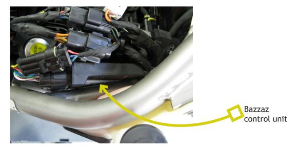
4. Connect the Bazzaz fuel harness to the control unit and begin routing the harness following along the factory harness towards the tail. The section of the Bazzaz harness with the injector connectors and TPS connector will back-track forward and into the airbox, following the factory harness; the section of the harness with the CKPS and neutral connectors routes around the rear of the airbox.
