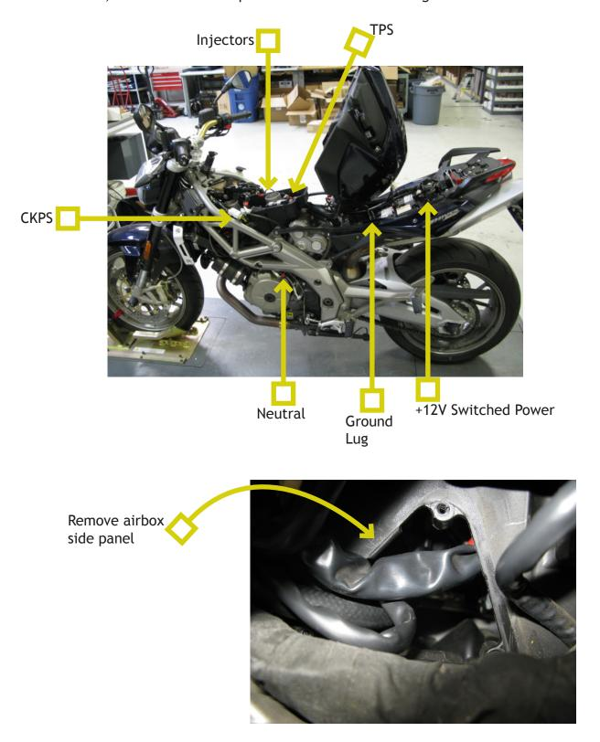
2. Next you will need to remove the top bracket that is secured between the front and rear throttle bodies. This will give you access to the injectors.
