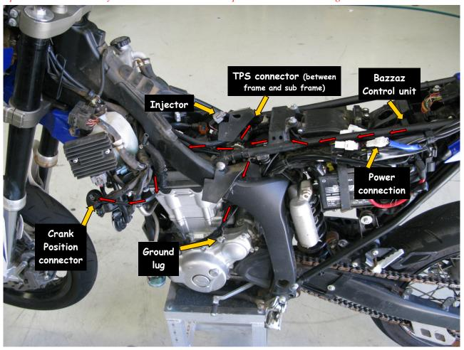
Note: Photo serves as a reference for the general location of component connectors that are required to be accessed throughout the installation. Please refer to your service manual for exact component locations. <u>Red arrows</u> simulate recommended harness routing.
