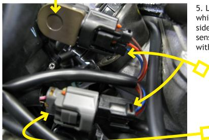
5. Locate the factory Throttle Position Sensor (**TPS**), which will be found on the rear throttle body (left side). Disconnect the factory TPS connector from the sensor and install the Bazzaz TPS connectors in-line with the factory connector and sensor.
