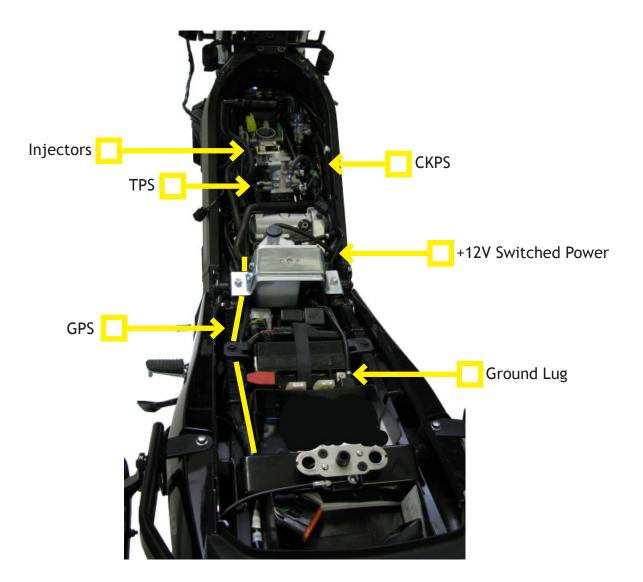
3. Route the Bazzaz **GROUND LUG** lead towards the negative battery terminal. Install the ground lug to the negative battery terminal.
