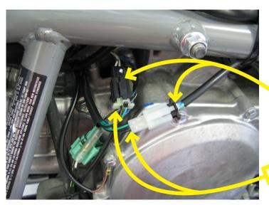
6. Route the remaining portion of the Bazzaz fuel harness down the left side of the frame and locate the black factory Crank Position Sensor (CKPS) connectors. Disconnect the factory CKPS connectors and connect the Bazzaz CKPS connectors in-line with the factory connectors.
