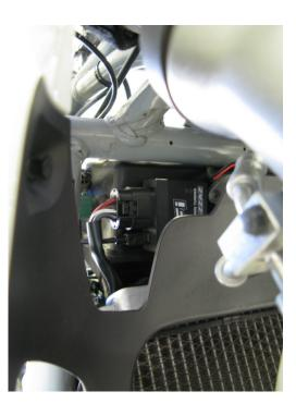
3. Now connect the main connector of the Bazzaz **FUEL HARNESS** to the control unit and begin routing the harness back towards the engine, on the right side of the scooter.
