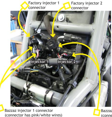
Bazzaz injector 2 connector (connector has red wires)
