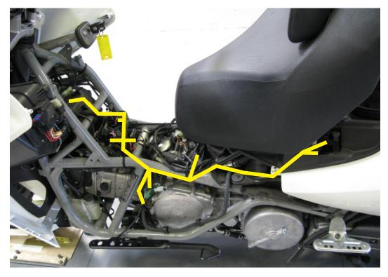
4. Route the fuel harness across the back of the motor and locate the **INJECTORS**. From right (injector 2) to left (injector 1), disconnect the factory injector connectors from each injector and install the Bazzaz injector connectors in-line, between the factory connectors and injectors.
