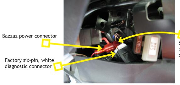
Scotchlok crimped onto the orange/white wire of the diagnostic connector
