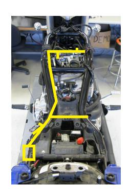
3. Route the Bazzaz power lead (orange sticker) back to the factory tail light connector, located along the frame on the left side of the motorcycle. Locate the large **gray** wire from the factory tail light connector and crimp a supplied scotchlok onto it. Now insert the Bazzaz power connector (red connector with red wire) into the scotch lok.
