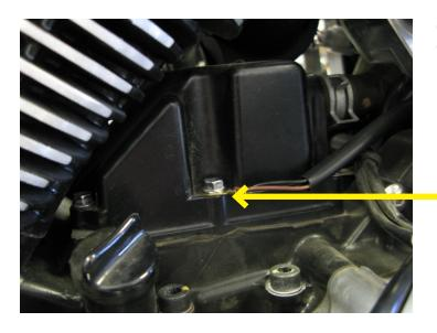
6. Attach the Bazzaz ground lug to a suitable chassis ground.
