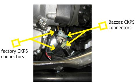
5. Now route the Bazzaz GPS connectors through the space behind the engine, to the right side of the motorcycle. Locate the factory GPS connectors (white connectors) and plug the Bazzaz GPS connectors inline with the factory connectors.
