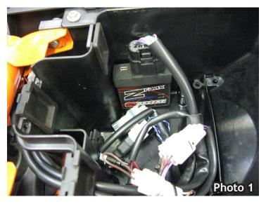
3. Route the harness out of the accessory box using the access slot on the left side (photo 2).
