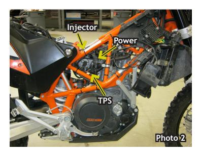
4. Identify the injector connector which can be found at the top of the throttle body assembly. Disconnect the factory harness connector and install the mating Bazzaz harness injector connectors inline (photo 3).
