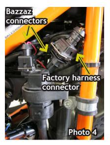
6. Disconnect the factory harness throttle position sensor connectors from the sensor and install the mating Bazzaz harness connectors inline (photo 5).
