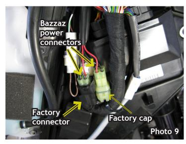
Prior to reinstalling the right side air inlet duct, route the remainder of the Bazzaz harness containing the control module connector toward the front of the motorcycle into the nose fairing (photo 10). Connect mating Bazzaz harness connectors to the control unit. Reinstall the right air inlet duct and secure the Bazzaz control module to the front of the air duct using the Velcro strips and long cable ties provided with the kit (photo 11).
