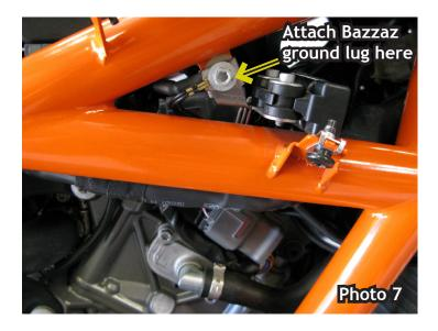
6. Near the factory ECU there is a black four pin connector with a dummy plug inserted into it on the factory harness. Remove the dummy plug and connect the mating Bazzaz power connector into this factory connector and insert the dummy plug into the remaining mating Bazzaz power connector (photos 8 & 9).
