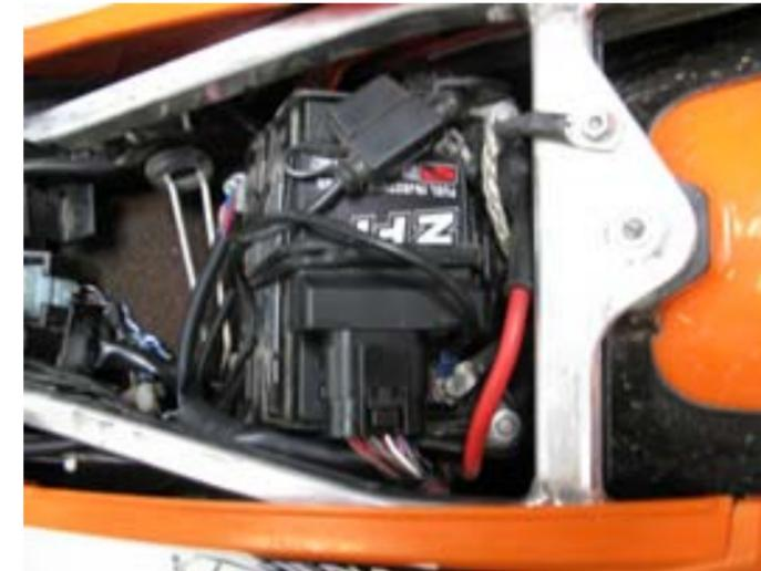
3. Connect the main connector of the Bazzaz **FUEL HARNESS** to the control unit. Begin routing the harness forward, towards the engine on the left side of the subframe and airbox cover. Continue to route the harness between the frame and the throttle body.
