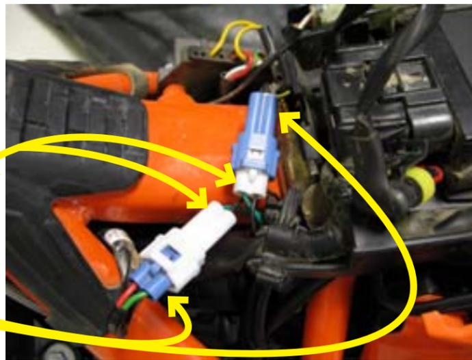
5. Next, locate the factory TPS, which is found directly on the left side of the throttle body and has a three pin connector at the end of the lead. Disconnect the three pin factory TPS connectors and install the Bazzaz **TPS** connectors in-line with the factory connectors.
