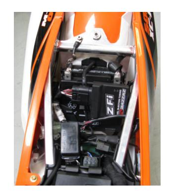
3. Connect the Bazzaz fuel harness to the control unit. Begin routing the harness forward, towards the engine on the left hand side, between the air box and the sub frame. Locate
