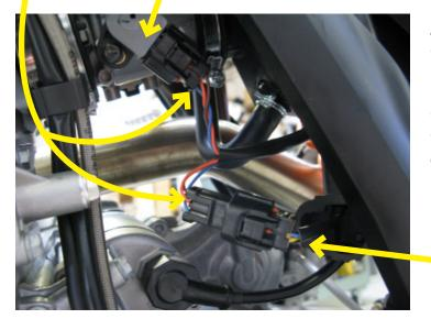
4. Now route the fuel harness inside the frame towards the engine. Locate the factory Throttle Position Sensor (TPS), which can be found on the lower left hand side of the throttle body. Disconnect the TPS connector from the sensor and connect the Bazzaz TPS connectors in line with the factory connector & sensor.
