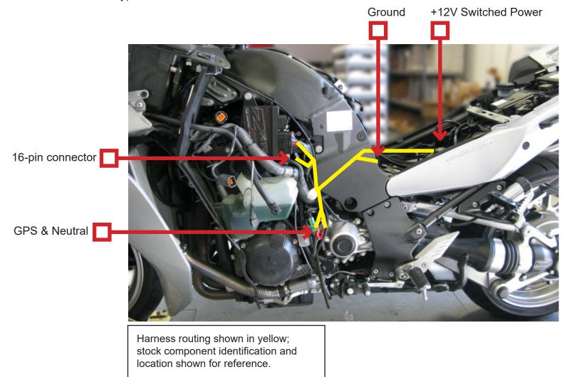
2. Connect the main connector of the Bazzaz **FUEL HARNESS** to the control unit. Locate the large, brown factory 16-pin connectors inside the engine compartment, behind the cylinders. These connectors contain the signal wires for the injectors, crank position sensor (CKPS) and throttle position senor (TPS). Disconnect the factory 16-pin connectors and connect the Bazzaz **16-PIN CONNECTORS** in-line with the factory connectors.
