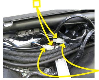
5. Locate the factory brake switch connectors on the right side of the under-seat area. Disconnect the factory brake switch connectors and plug the Bazzaz **+12V SWITHCED POWER** connectors in-line with the factory connectors.
