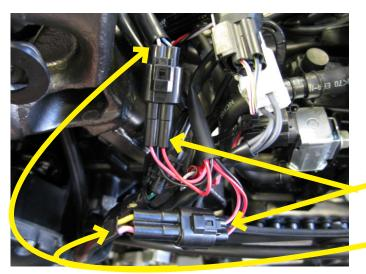
3. Route the harness down the right side of the bike towards the engine. Locate the factory three-pin, black speed connectors which can be found near the factory fuel pump connector (on the left side of the bike). Disconnect the factory speed connectors and connect the Bazzaz **SPEED** connectors in-line with the factory connectors.
