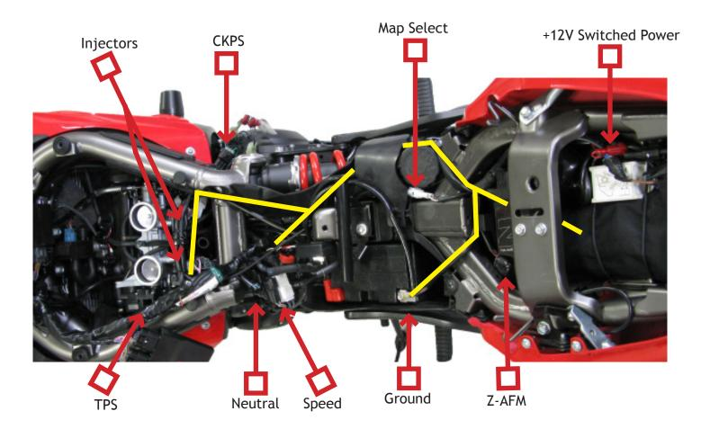
2. Mount the **CONTROL UNIT** on top of the tool kit using the tool kit straps. Connect the main connector of the Bazzaz **FUEL HARNESS** to the control unit.
