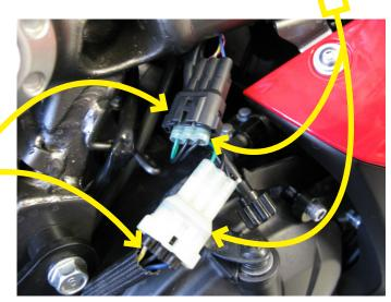
6. Route the Bazzaz injector connectors to the factory injectors which can be found directly beneath the factory fuel rail.
