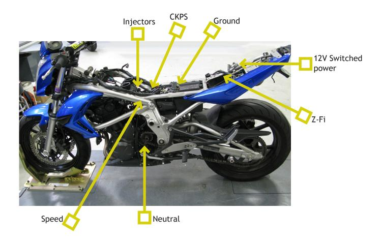
2. Place the control unit in the tail of the motorcycle and secure it using the supplied velcro patch. Connect the main connector of the fuel harness into the control unit and begin routing the fuel harness over the top of the sub-frame and down along the factory harness.
