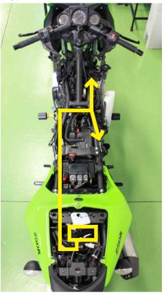
3. Locate the factory tail light connectors in the tail section of the bike and disconnect them. Connect the +12V switched power connectors of the Bazzaz fuel harness inline with the factory connectors.
