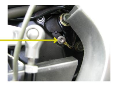
5. Continue to route the fuel harness along with the factory harness, forward to the Throttle Position Sensor (TPS) sensor which is located on the left side of the throttle bodies. Unplug the factory TPS connector and plug the Bazzaz TPS connectors inline between the factory connector and sensor.
