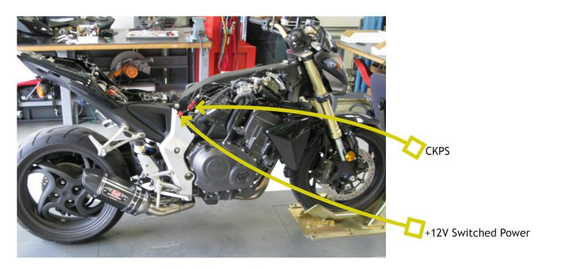
2. Place control unit in the tail of the motorcycle and connect the fuel harness main connector to the control unit. Begin by routing the harness to the left of the battery. The main section of the harness will continue to route along the left side of the motorcycle, while the section containing the CKPS and power connectors will route to the right side of the motorcycle.
