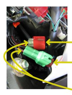
8. Next Locate the red diagnostic connector with a red cap on it. Remove the cap and plug the Bazzaz +12V switched power lead into the connector, replacing the cap onto the other side of the Bazzaz clear power connector.
