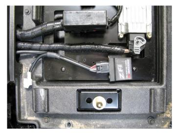
3. Connect the main connector of the Bazzaz **FUEL HARNESS** to the control unit. Begin routing the harness along the same path as the factory harness, into the center console, and then back towards the engine (as shown in photo above).
