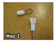
The Bazzaz control unit is capable of storing two maps. These maps can be selected by connecting or disconnecting the map select jumper on the fuel harness (or you can switch maps on the fly with the handle bar mounted map select switch, sold separately). When the map select jumper is connected, the control unit is operating using map 1. When the map select jumper is disconnected, the control unit is operating using map 2.
