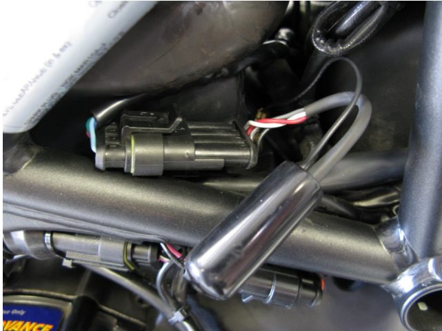
Front Cylinder O2 eliminator
