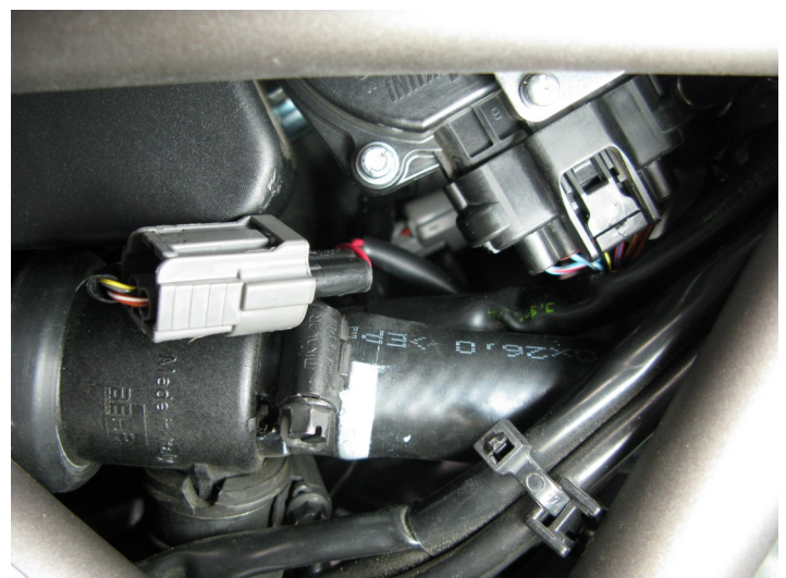
Bazzaz harness installed in-line
