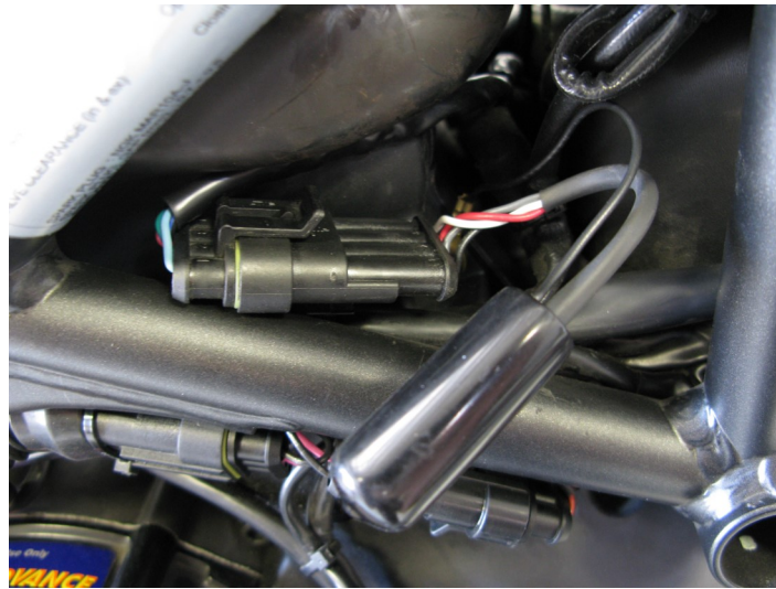
Bazzaz O2 Stabilizer installed
