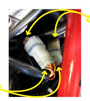
Factory secondary fuel injector connectors
