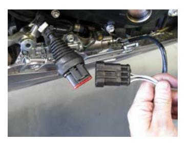
The Bazzaz control unit is capable of storing two maps. These maps can be selected by connecting or disconnecting the map select jumper on the fuel harness (or you can switch maps on the fly with the handle bar mounted map select switch, sold separately). When the map select jumper is connected, the control unit is operating using map 1. When the map select jumper is disconnected, the control unit is operating using map 2.
