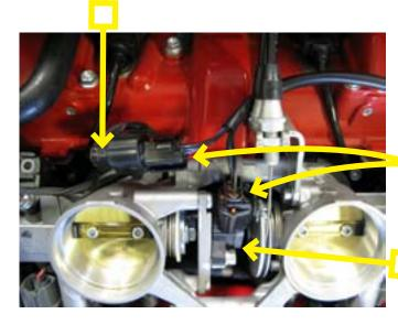
9. Route the remaining fuel harness up the right side of the throttle bodies and around the front, to the factory Throttle Position Sensor (TPS). Disconnect the factory TPS connector from the sensor and connect the Bazzaz **TPS** connectors in-line with the factory sensor and connector.
