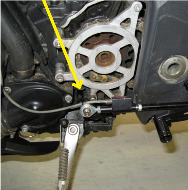
scotchlok crimped onto the factory black/white wire
