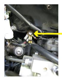
5. Next locate the factory ground lug and attach the Bazzaz ground lug to it.
