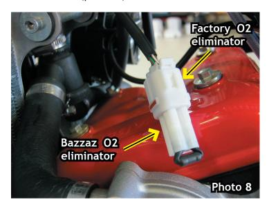
10. Now that the installation is complete, take a moment to secure the Bazzaz harness along its routing path with the supplied cable ties. Reinstall the components removed in step one of these instructions.
