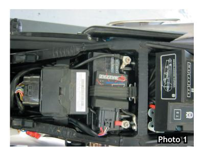
3. Plug the main connector into the Bazzaz unit and proceed to route the harness forward, following the stock harness under the main frame rail (photo 2).
