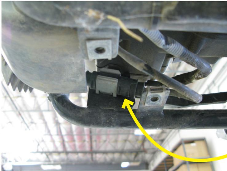
8. Now you will need to eliminate the factory **O2/ LAMBDA SENSOR**, as this sensor will no longer be used. The sensor connector is a round four-pin connector, found attached to the right side of the frame and under the skid plate. Simply disconnect the connectors; the wires should be neatly secured away from any moving components, or the sensor may be removed and the remaining port/bung in the exhaust can then be plugged.
