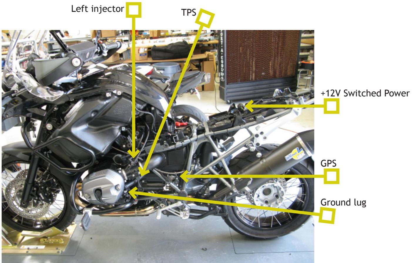
2. Mount the control unit under the tank, against the fuse box using the supplied Velcro patch. Connect the fuel harness main connector to the control unit. Route the portion of the fuel harness with the right side injector and CKPS connector through to the right side of the bike. Route the portion with the GPS and +12V switched power connector toward the rear of the bike and next to the battery. The remaining portion can hang on the left side for now.
