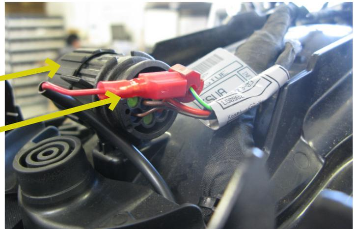
8. Route the right side injector connectors under the air intake tube to the injector on top of the throttle body. Disconnect the factory injector connector and plug the Bazzaz connectors in line between the factory connector and injector.
