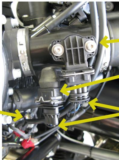
5. Route the Bazzaz fuel harness ground lug past the TPS and attach it at one of the bolts on the side of the cylinder; we recommend using the same bolt that the coils' ground wire goes to.
