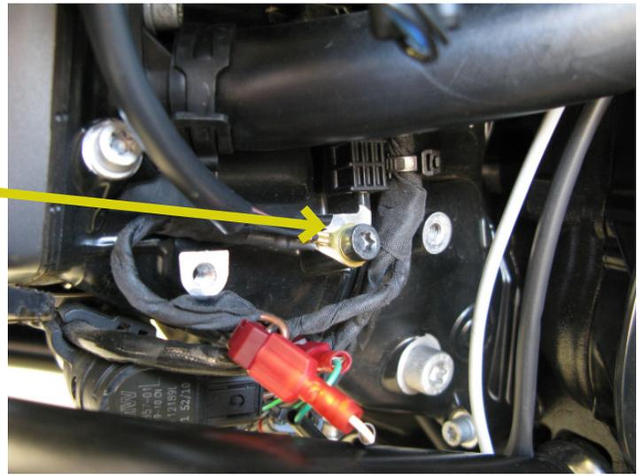
6. Next route the Bazzaz GPS connector down to the factory GPS connector, found just in front of the rear wheel, behind the exhaust servo (moved out of the way in step 1). Crimp a supplied scotchlok onto the middle **purple/black** wire of the factory GPS connector, and insert the Bazzaz GPS connector (red connector with pink wire) into the scotchlok.
