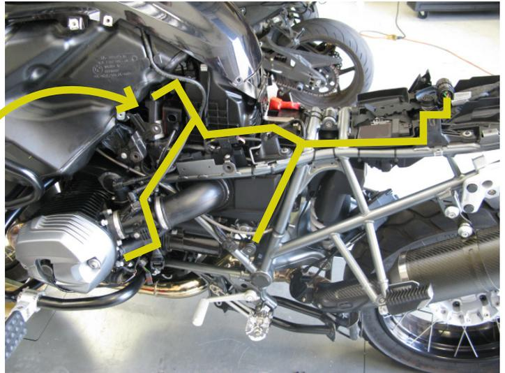
3. Locate the left side injector, on top of the throttle body. Unplug the factory injector connector and plug the Bazzaz injector connectors in line between the factory connector and injector.
