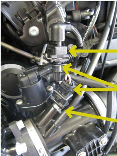
4. Locate the TPS connector, just below the left side injector. Unplug the factory connector and plug the Bazzaz connectors in line between the factory connector and the TPS.
