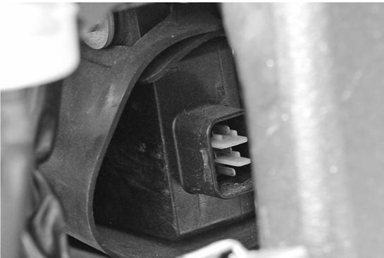
3 Connect the Bazzaz EXUP eliminator to the factory wiring harness in place of the servo motor. Secure the wiring in a suitable location using the provided velcro strip.
