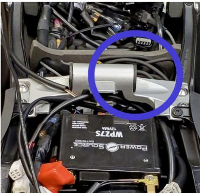
2. Unplug the servo connector. Remove the EXUP servo from the motorcycle.
