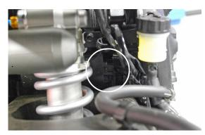
2. Unplug the servo connector. Remove the EXUP servo from the motorcycle.
