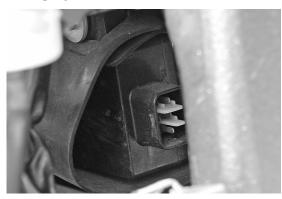
3 Connect the Bazzaz EXUP eliminator to the factory wiring harness in place of the servo motor. Secure the wiring in a suitable location using the provided velcro strip.
