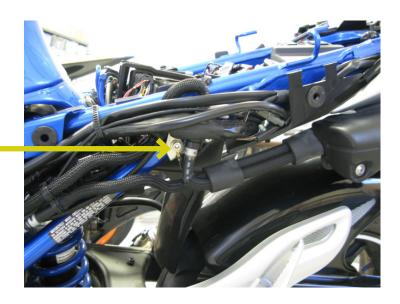
6. Locate Gear Position Sensor connector, on the left side of the engine compartment just forward of the Throttle Position Sensor, and install the Bazzaz GPS connectors in line with the factory connectors.
