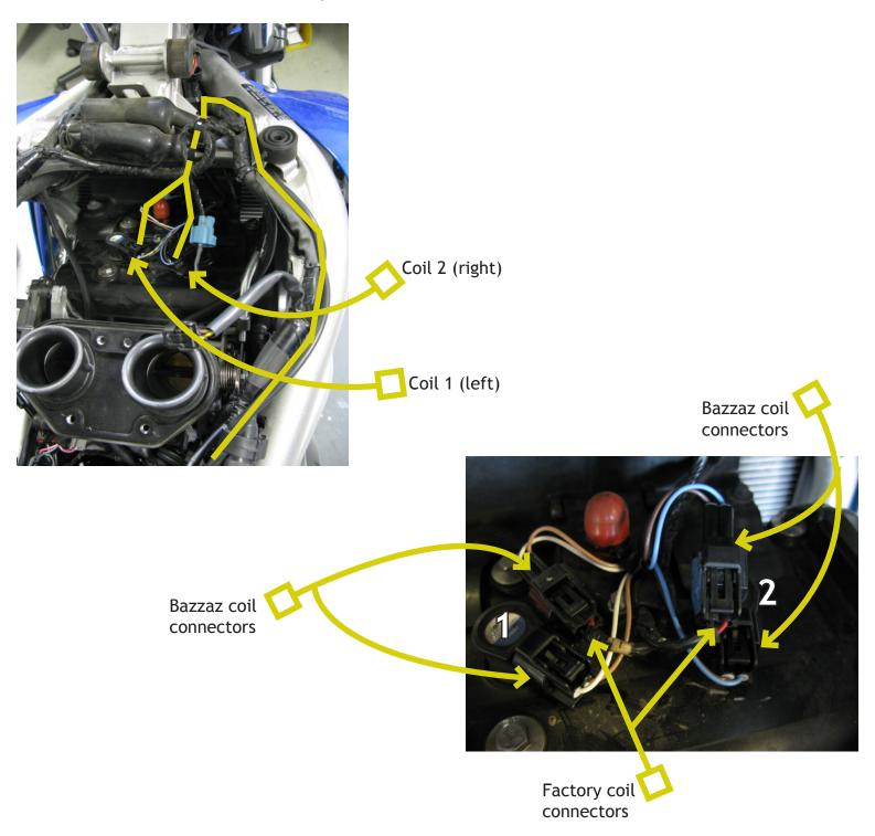
11. In order to install the quickshiftter, aftermarket rearsets must be used. Install the **SHIFT SWITCH** (installation of shift switch will vary depending on brand of rearsets), and then route the shift switch connector to the mating connector on the Bazzaz coil harness and connect.
