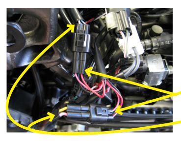
3. Route the harness down the right side of the bike towards the engine. Locate the factory three-pin, black speed connectors which can be found near the factory fuel pump connector (on the left side of the bike). Disconnect the factory speed connectors and connect the Bazzaz **SPEED** connectors in-line with the factory connectors.
