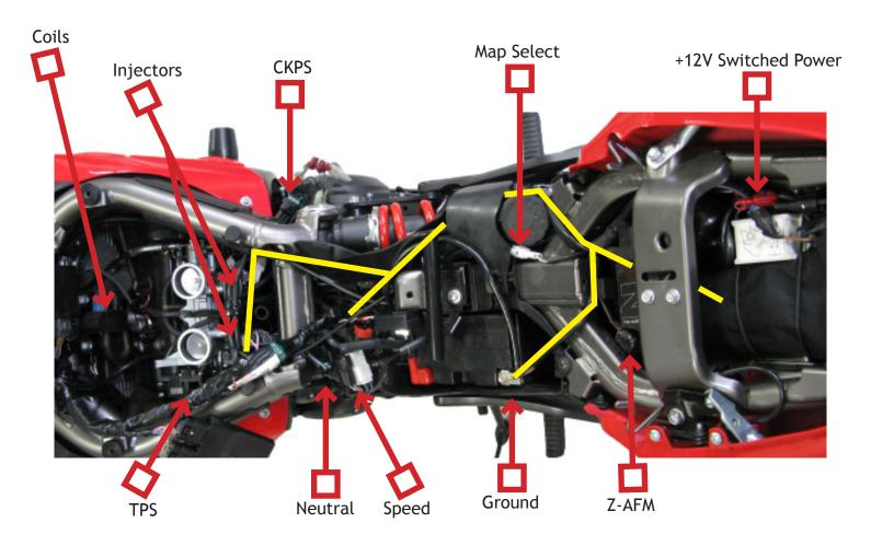
2. Mount the **CONTROL UNIT** on top of the tool kit using the tool kit straps. Connect the main connector of the Bazzaz **FUEL HARNESS** to the control unit.
