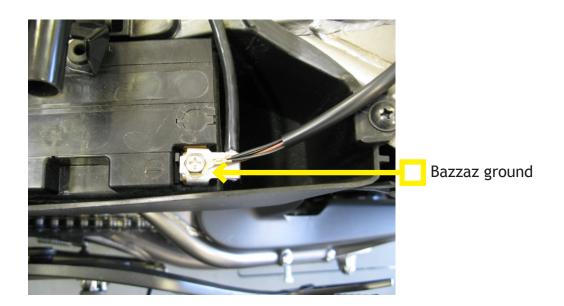
10. Now, connect the main connector of the Bazzaz COIL HARNESS to the control unit and begin to route the coil harness along the right side of the bike, up to the valve cover. Disconnect the factory coil connectors from each coil and plug the Bazzaz COIL connectors (right to left) in-line with the factory coil and coil connector. The Bazzaz coil connectors with the blue and brown wires will go to coil #2 (right coil).
