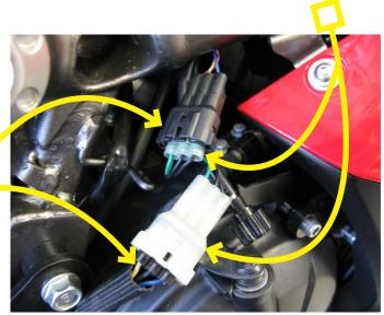
6. Route the Bazzaz injector connectors to the factory injectors which can be found directly beneath the factory fuel rail.
