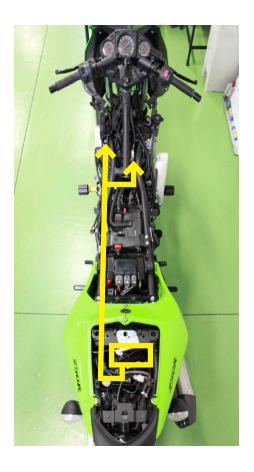
13. Locate the factory coil connectors. Disconnect the factory coil connectors from the ignition coils and connect the Bazzaz coil connectors inline with them according to the labels.
