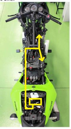
3. Locate the factory tail light connectors in the tail section of the bike and disconnect them. Connect the +12V switched power connectors of the Bazzaz fuel harness inline with the factory connectors.
