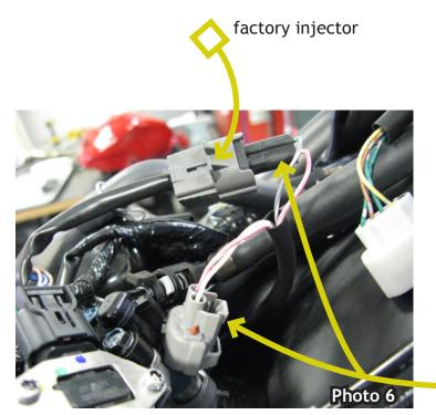
7. Route the remainder of the harness to the front of the bike and locate the factory injector on the top of the throttle body. Plug inline with the Bazzaz injector (photo 6).
