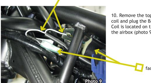
10. Remove the top spade connector from the factory coil and plug the Bazzaz coil spade connectors inline. Coil is located on the upper frame rail underneath the airbox (photo 9).
