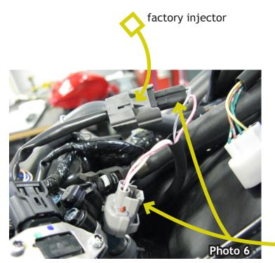
7. Route the remainder of the harness to the front of the bike and locate the factory injector on the top of the throttle body. Plug inline with the Bazzaz injector (photo 6). 8. Now locate the factory +12V switched power and plug the Bazzaz +12V switch (orange tag) inline. Connector located at the front of the bike close to the coil, under the air box (photo 7).
