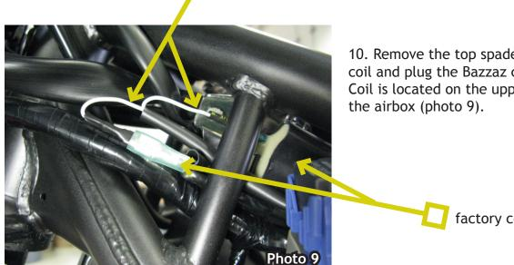
10. Remove the top spade connector from the factory coil and plug the Bazzaz coil spade connectors inline. Coil is located on the upper frame rail underneath the airbox (photo 9).
