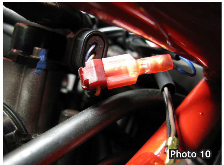
Bazzaz TPS lead installed
