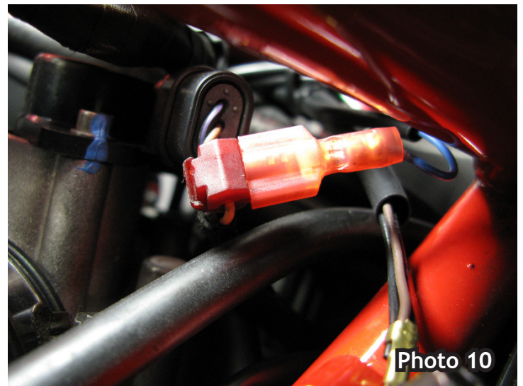
Bazzaz TPS lead installed
