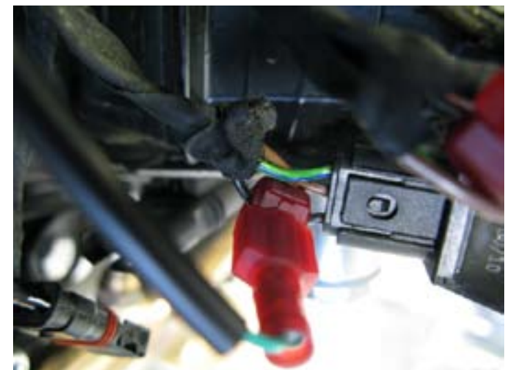
Coil right side (black signal wire with yellow tracer)
