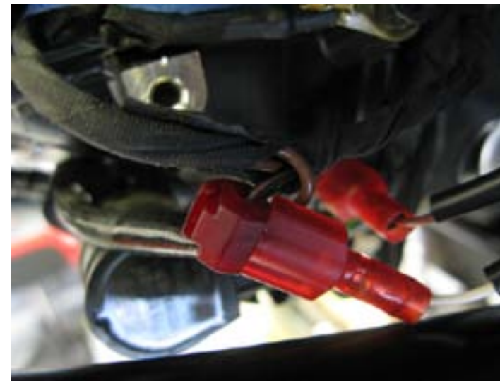
Coil left top (black signal wire with brown tracer)
