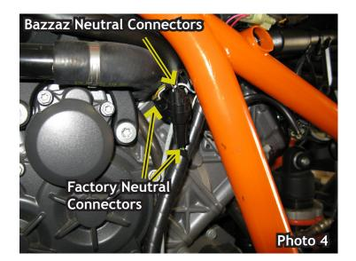
6. Once again disconnect the factory harness from the ignition coil for the rear cylinder and connect the mating Bazzaz coil connector inline (photo 5).
