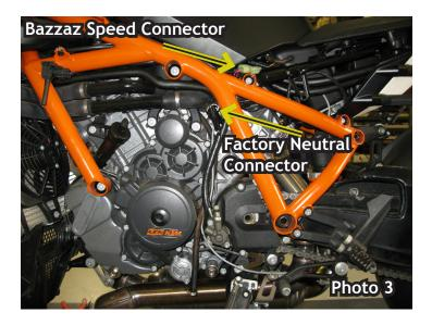
5. Disconnect the factory connectors and install the mating Bazzaz neutral sensor connectors inline (photo 4).
