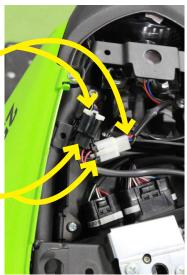
4. Locate the factory speed sensor connectors on the left side of the bike just before the main frame rail and disconnect them. Connect the Bazzaz speed sensor connector's in-line with the factory connectors.
