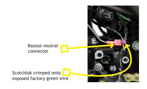
Drive sprocket cover will need to be removed to gain access.
